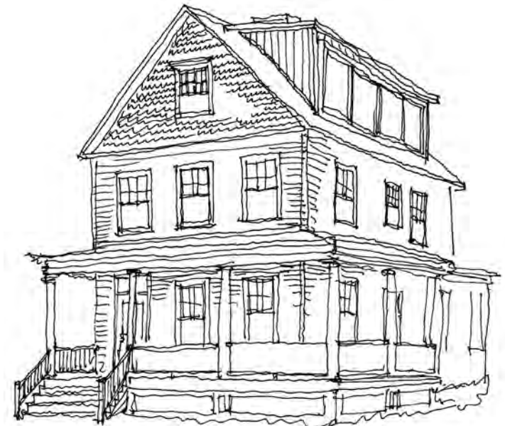
Not recommended: Dormers that occupy a high percentage of the existing roof area and introduce new forms to the building.
