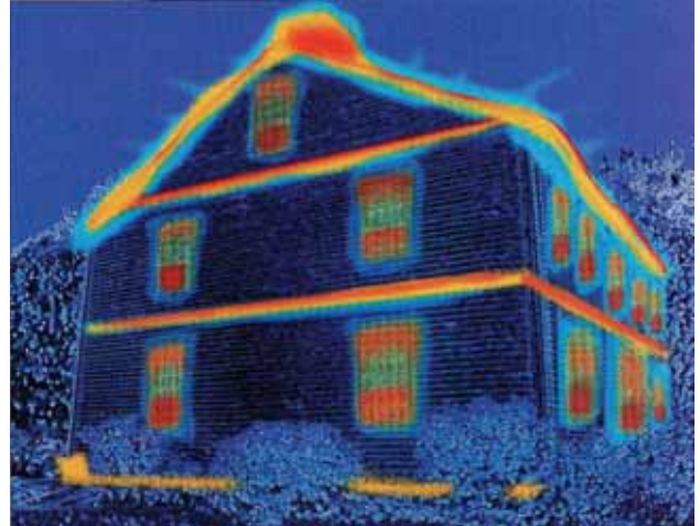
New techniques like infra-red photography highlight heat leaks and help builders make old and historic buildings energy efficient while retaining character.
